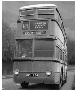
Above: London Transport's Q5 was a Country Area bus and therefore had a centre entrance and sliding door. The Central Area Q double-deckers had open front platforms. The Q5 must have looked resplendent in its green and black pre-war livery. (H Snook)
