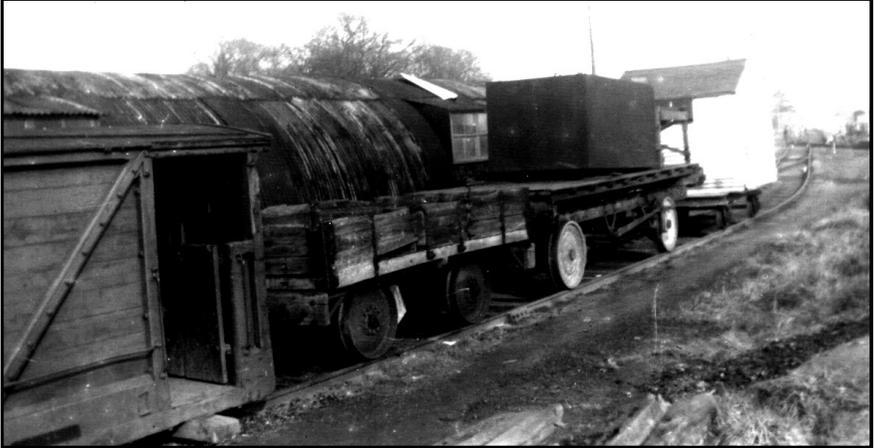
While sorting out some papers, I came across the above photograph, taken during the SLS Railtour to the Shropshire & Montgomeryshire on 20 March 1960. The location is the siding behind the Nissen hut at Kinnerley. The picture shows the light 4-wheeled baggage trailer purchased to run with the Ford railmotor set, but rarely used.
